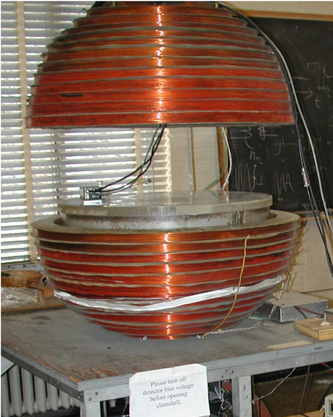
Figure A-2: A fluxball of Clark's design is still operated by the Physics Department at the Massachusetts Institute of Technology.
